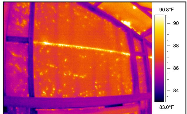
Figure 5. Thermal image of beetle damaged end wall insulation.
