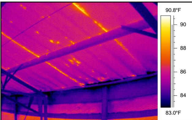
Figure 4. Thermal image of beetle damaged ceiling insulation.
