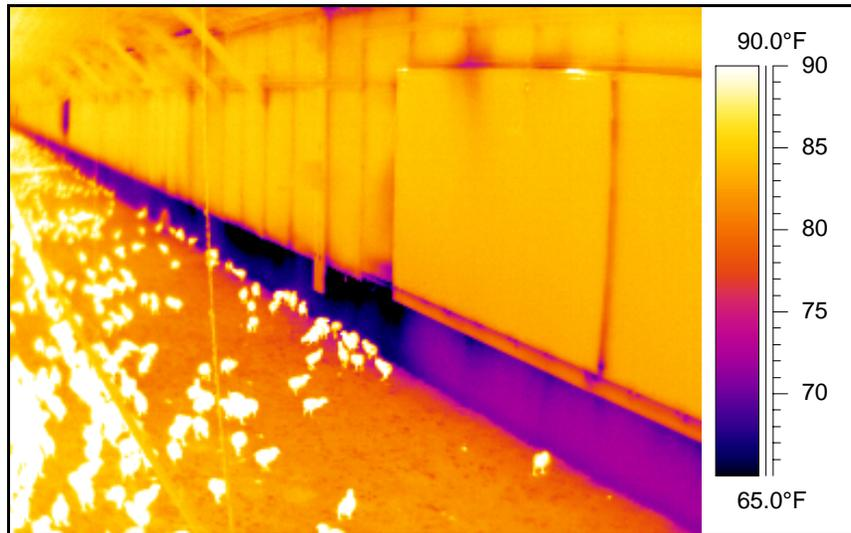
Air leakage due to beetle damaged sill sealer in background. The sill in the foreground was caulked to eliminate leakage.
